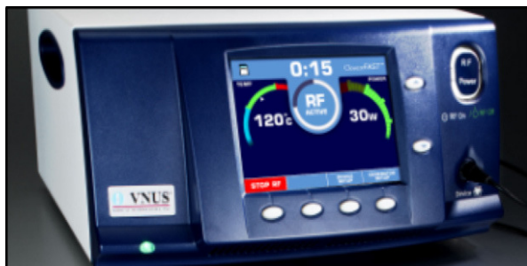
Fig. 4 – RFG2 Plus generator TM . The control unit display shows the real time power, temperature and treatment cycles.
