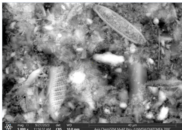
Fig. 4 – SEM image of a diatomite sample heat treated at 700 °C, magnification 5000×.
