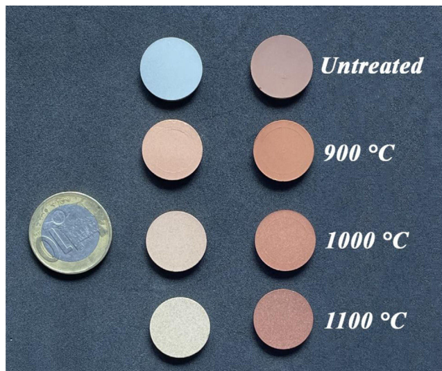
Fig. 7 – Color change of ceramic membranes sintered at different temperatures.
