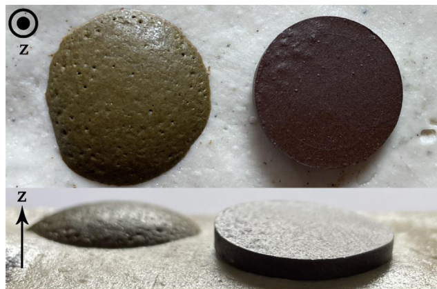
Fig. 8 – Appearance of clay pellets after thermic treatment at 1170 °C.
