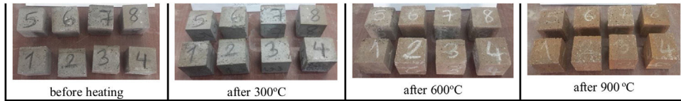
Fig. 8 – Visual appearance of geopolymer specimens before heating and after 300 °C, 600 °C, and 900 °C heating.
