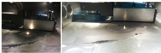
Fig. 3.1 – Powder with bad (left) and good (right) flowability.
