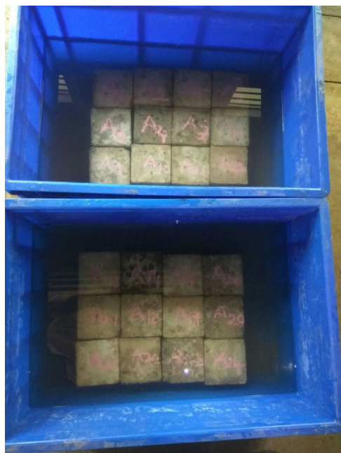
Fig. 11 – Specimens immersed for water absorption test.
