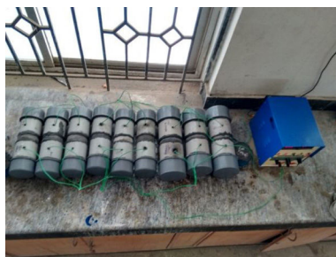
Fig. 10 – Specimens casted for RCPT.
