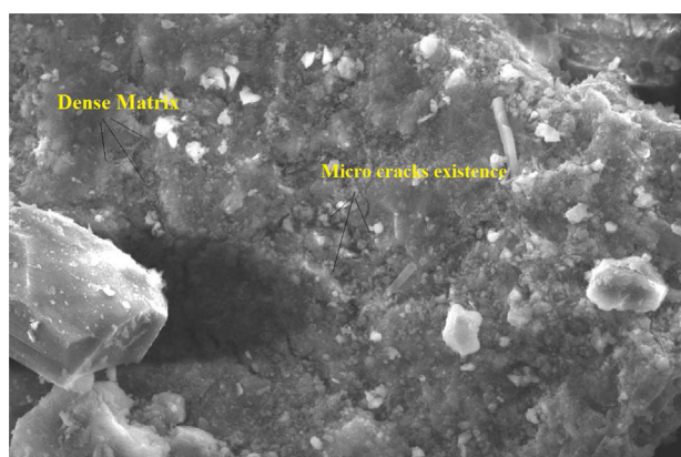
Fig. 17 – SEM image of GPC after 12 months of immersion in sulphate solution.
