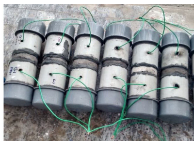
Fig. 10 – Specimens casted for RCPT.
