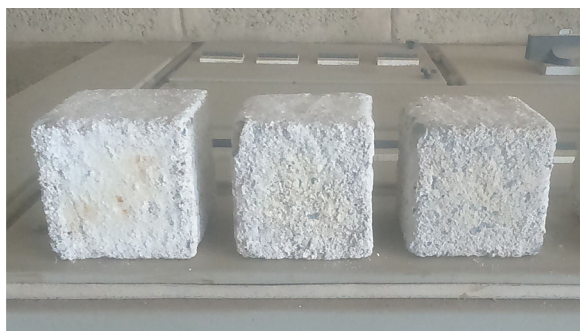
Fig. 18 – Visual appearance of GPC specimens after Immersion in sulphuric acid solution.
