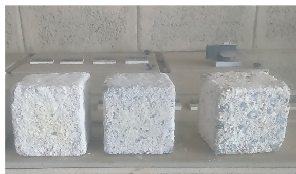
Fig. 19 – Visual appearance of CC specimens after Immersion in sulphuric acid solution.
