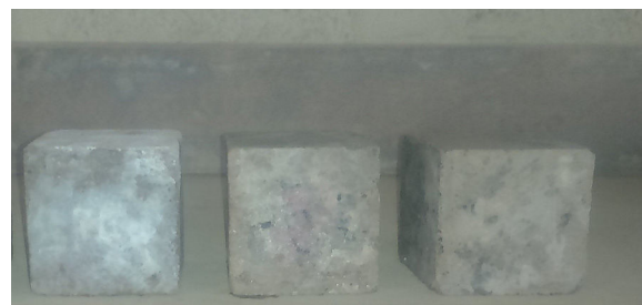
Fig. 13 – Visual appearances of CC specimens after immersion in magnesium sulphate solution.
