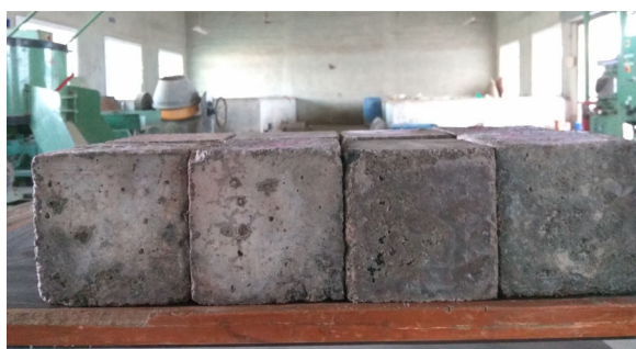
Fig. 12 – Visual appearances of GPC specimens after immersion in magnesium sulphate solution.
