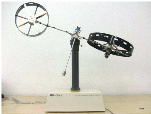
Figura 1: Twin Rotor MIMO System (TRMS) modelo 33-220.
