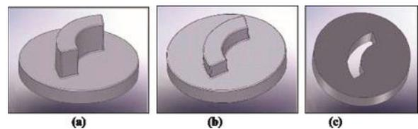
Fig. 8. Design of die for simulation (a) lower puncture (b) upper puncture (c) cavity.
