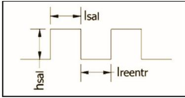
Fig. 3. Rotor topology in the horizontal plane.
