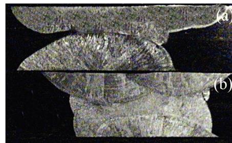
Fig. 2. Macrostructure of weld joints produced (a) ERNiCrMo-3 PCGTAW and (b) ERNiCrMo-4 PCGTAW.
