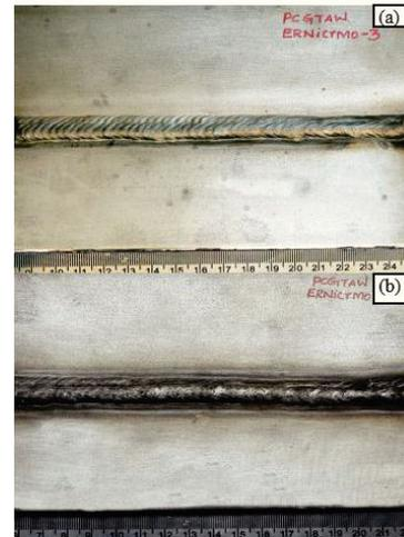
Fig. 1. Photographs of weld joints (a) ERNiCrMo-3 PCGTAW and (b) ERNiCrMo-4 PCGTAW.
