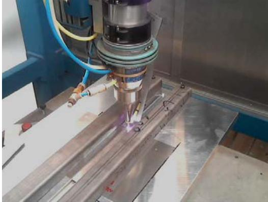
Fig. 4. Welding process at initial moment.
