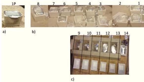
Fig. 6. Moulds submitted to heat treatment: a) cycle 1, b) cycle 2 and c) cycle 3, after casting.
