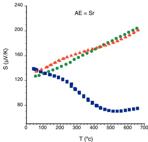
**Fig. 6 – Temperature dependence of the Seebeck coefficient of  $\text{Bi}_2\text{Sr}_2\text{Co}_{1.8}\text{O}_x$  samples, as a function the processing method: ● solid state sintered, ■ LFZ as-grown and, ▲ LFZ annealed.**
