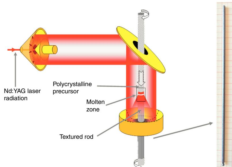
**Fig. 1 – Schema of the laser floating zone system used in this work. A typical as-grown Bi-AE-Co-O sample is shown in the right side of the figure.**
