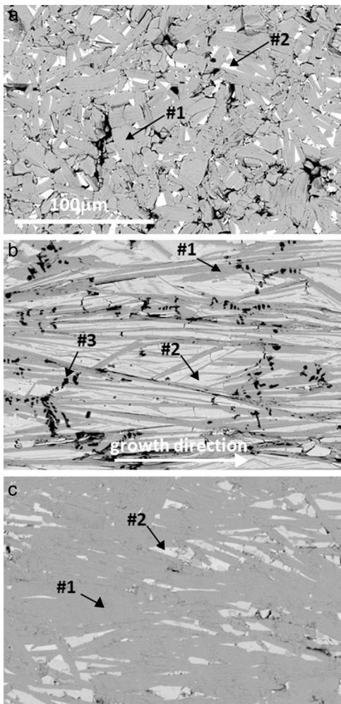
**Fig. 4 – Typical FESEM (backscattered electrons) micrographs of Bi-AE-Co-O (AE = Ca) longitudinal polished sections: (a) solid state sintered, (b) LFZ as-grown (the growth direction is specified by an arrow), and (c) annealed laser-textured. Different contrasts are #1: grey one, associated to the thermoelectric  $\text{Bi}_2\text{Ca}_2\text{Co}_{1.7}\text{O}_x$  phase; #2: light grey,  $\text{Bi}_6\text{Ca}_4\text{O}_{13}$ ; and #3: black, Co-oxide.**
