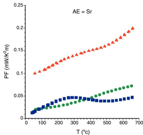
**Fig. 7 – Variation of PF with temperature for  $\text{Bi}_2\text{Sr}_2\text{Co}_{1.8}\text{O}_x$  samples, as a function the processing method: ● solid state sintered, ■ LFZ as-grown and, ▲ LFZ annealed.**
