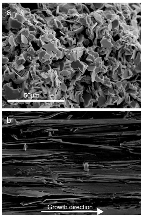
**Fig. 3 – Typical FESEM (secondary electrons) micrographs of  $\text{Bi}-\text{AE}-\text{Co}-\text{O}$  ( $\text{AE} = \text{Ca}$ ) fractured surfaces: (a) solid state sintered, and (b) LFZ as-grown (the growth direction is specified by an arrow).**
