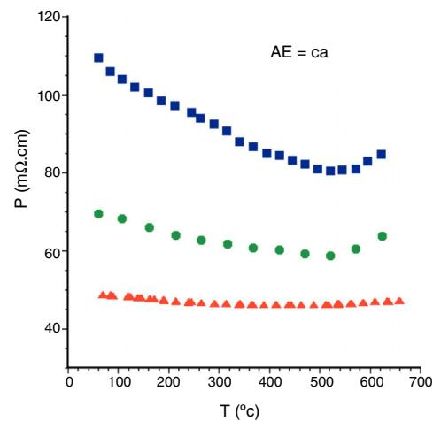
**Fig. 5 – Temperature dependence of the electrical resistivity of  $\text{Bi}_2\text{Ca}_2\text{Co}_{1.7}\text{O}_x$  samples, as a function the processing method: ● solid state sintered, ■ LFZ as-grown and, ▲ LFZ annealed.**
