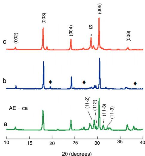
**Fig. 2 – Powder XRD patterns of the different  $\text{Bi}_2\text{Ca}_2\text{Co}_{1.7}\text{O}_x$  samples: (a) solid state sintered, (b) LFZ as-grown, and (c) LFZ annealed. Crystallographic planes indicate the peaks for the  $\text{Bi}_2\text{Ca}_2\text{Co}_{1.7}\text{O}_x$  TE phase (indexed as  $P2/m$  space group), ♦ indicates Co-free secondary phase indexed as  $\text{Bi}_6\text{Ca}_4\text{O}_{13}$  ( $Cmm2$  space group), and \* indicates the (111) Si peak, added as internal reference.**
