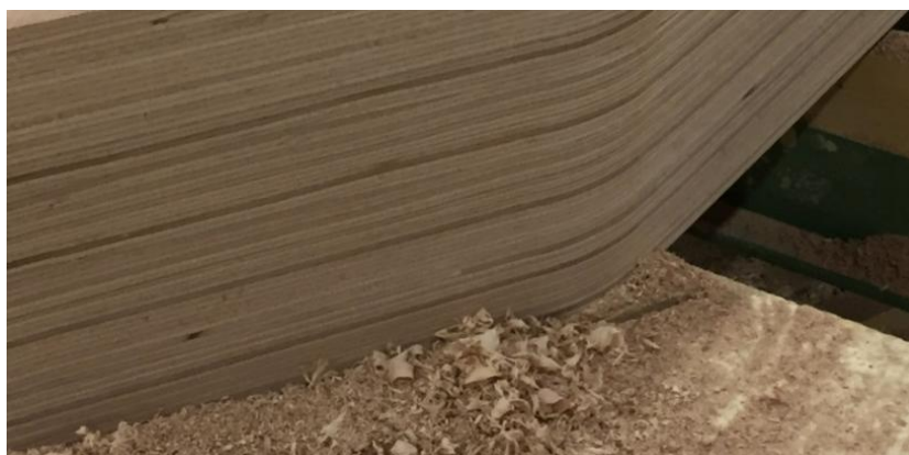
Figure 7. LVL Baubuche S showing distinctive 3mm laminations
